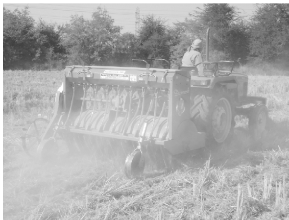
Fig. : 5 - Happy Seeder for direct drilling of seeds in presence of surface residue. (Photo courtesy CSISA, CIMMYT-IRRI, New Delhi)
